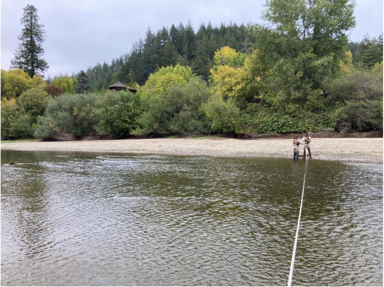
Figure A 14. A photo of the riffle crest transect taken at Vacation Beach on October 5, 2021
