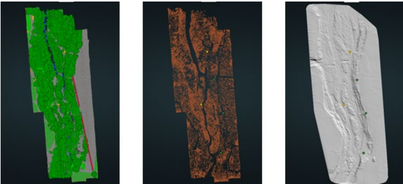
Data collected using drone with LiDAR sensor: riparian canopy layer (left panel), bare earth topographic points (middle panel), digital elevation model generated from bare earth points (right panel).
